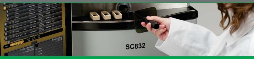
832 Series: Sulfur/Carbon Analysis by Combustion
